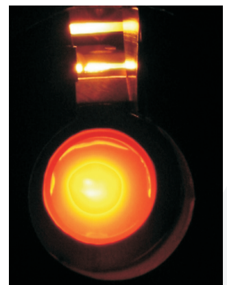
Look onto an EBVV evaporator with tilted hearth and additional Ta shielding parts (right hand under operation)
