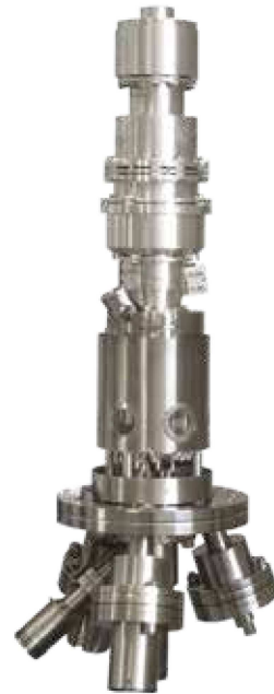
Photograph of the FERRUM spin-detector. The detector is mounted on a CF100 flange. Chamber and \mu -metal screens are removed for clarity.
