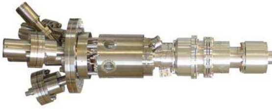
FIG. 2: Photograph of the FERRUM spin-detector. The detector is mounted on a CF100 flange. Chamber and \mu -metal screens are removed for clarity.
